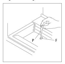
Frost is automatically eliminated from the evaporator of the refrigerator compartment every time the motor compressor stops, during normal use. The defrost water drains out through a trough into a special container at the back of the appliance, over the motor compressor, where it evaporates.
